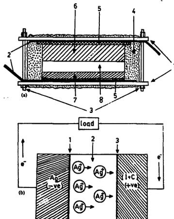
Fig. 1. (a) Cross-sectional view of solid-state primary battery with ebonite material: (1) ebonite sheets; (2) copper leads; (3) bolts and screws; (4) resin; (5) graphite sheets; (6) cathode pellet; (7) anode; (8) electrolyte. (b) Discharge process of silver-ion conducting, solid-state electrolyte cell: (1) anode and electrolyte interface; (2) silver-ion conducting electrolyte; (3) cathode and electrolyte interface.
