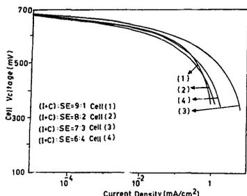
Fig. 5. Polarization characteristics of cells made of SSV glass with various cathode (I+C):SE compositions.
