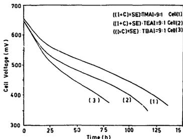
Fig. 8. Discharge characteristics of cells made of various cathode [(1+C)+SE]:TAAI (A = methyl, ethyl and butyl) compositions.
