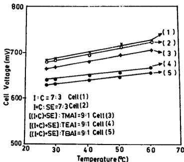
Fig. 2. Temperature dependence of open-circuit voltage of cells made up of SSV glass with various cathode materials I:C, (I+C):SE and [(I+C)+SE]:TAI (A = methyl, ethyl and butyl).
