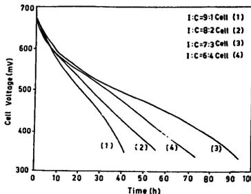
Fig. 4. Discharge characteristics of cells made up of various cathode I:C compositions; load = 100  $\mu\text{A cm}^{-2}$ .
