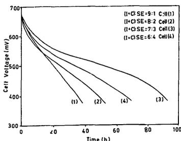
Fig. 6. Discharge characteristics of cells made up of various cathode (I+C):SE compositions; load =  $100 \mu\text{A cm}^{-2}$ .
