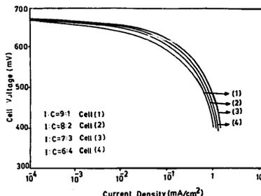
Fig. 3. Polarization characteristics of cells made up of SSV glass with various I:C compositions.
